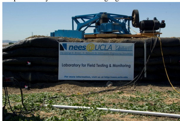
Figure 1. Model levee with MK-15 eccentric mass shaker mounted on crest.
