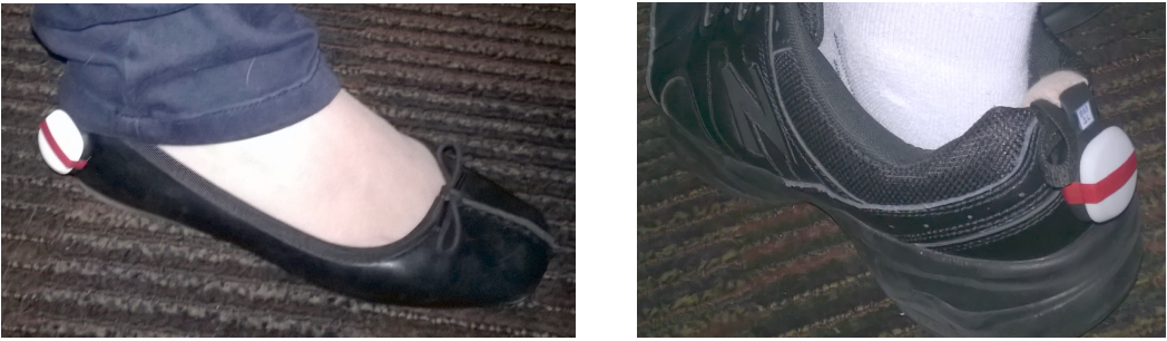
Fig. 3. Examples of placement of the CPRO shoe-mounted sensor for ground truth step detection. The sensor is contained in the white small case, attached to a plastic padded clip.
