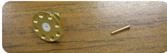
Figure 2.10: A Radiall 9003 connector was used for the SMA connector.
