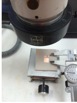
Figure 3.43: The actual dimensions of the parameters in the CP half E-shaped patch element were measured and compared with simulation data.
