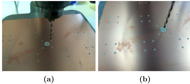
Figure A.3: The via holes for the SMA and the input pin of the SMA are drilled.
