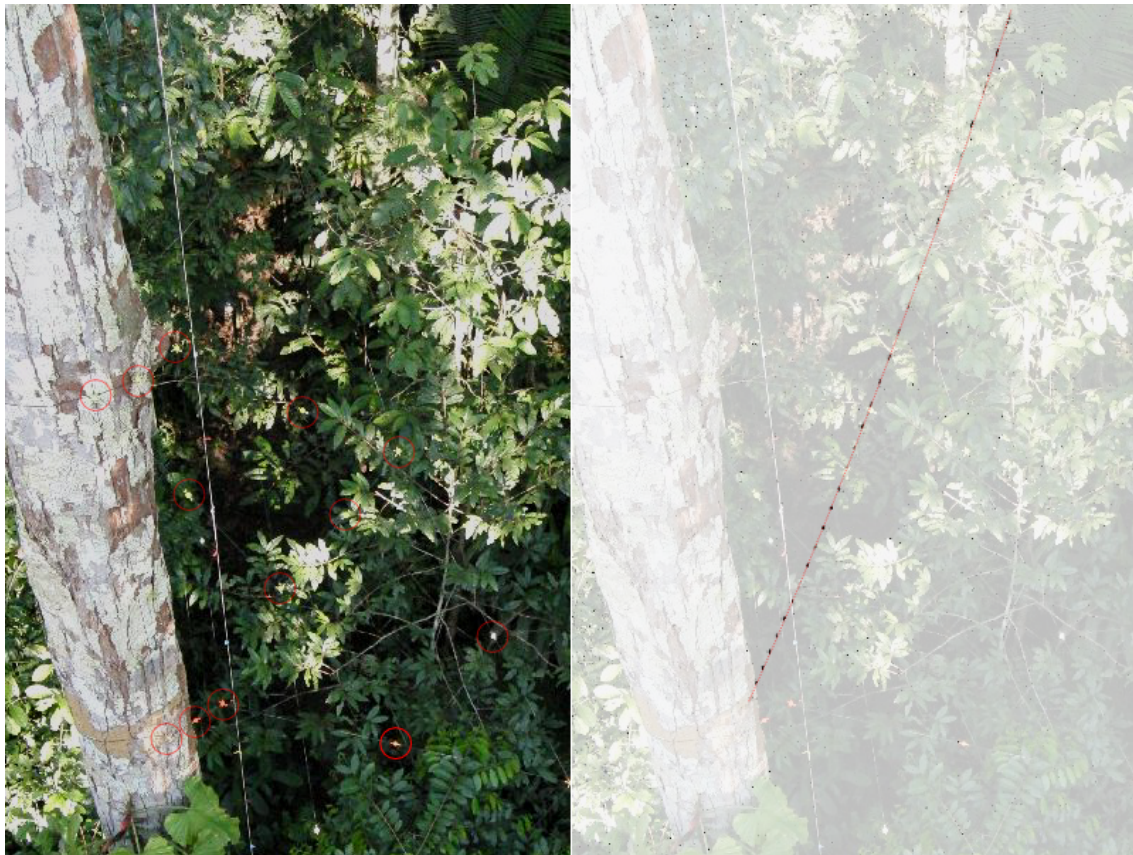
Figure 1.3: Left: Crop from raw video frame, showing forest background. Highlighted with red circles are the markers that comprise the calibration frame. Right: Composite image of a trial, showing ant position in successive frames. Spline interpolation is shown in red.
