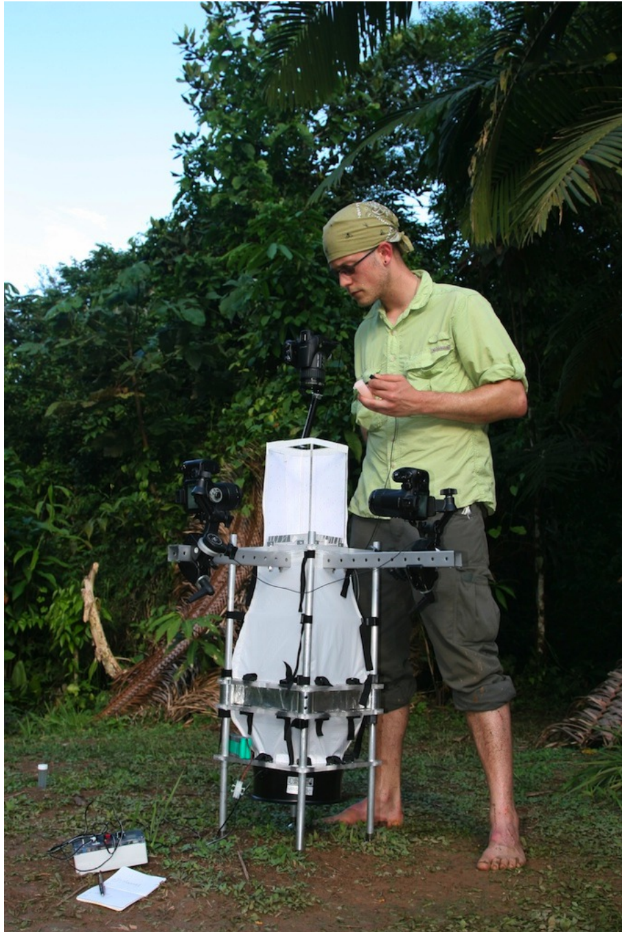
Figure 2.1: Photograph of portable wind tunnel used in this study, with 188 cm tall human provided for scale. Photo credit: Steve Yanoviak
