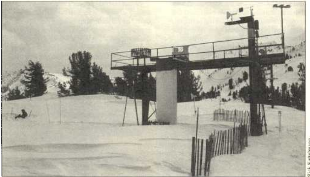
The SNARL snow science laboratory as seen from outside. The platform and top of the "Santa Claus tower" (center) are visible; the rest of the lab is buried within a seven-foot snowpack. On the far left, Reserve Manager Dan Dawson sits at the top of the snow sampling pit, recording data as a colleague measures snow density.
