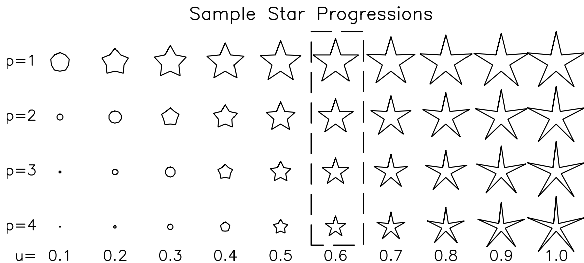
Figure 2: Progressions of star symbols corresponding to the variations of r and a shown in panels (a) through (d) of Figure 1, with the “perfect star” shape always being at u = 0.6 . Note that because the area of the circumscribing polygon varies as u^p , the radius varies as u^{p/2} ; so for p = 1 the radius varies as \sqrt{u} .
