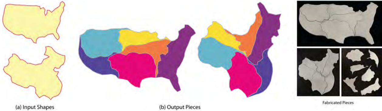
Figure 1.8: Given two input shapes (a), our Approximate Dissections approach generates a small number of pieces that may be arranged to form close approximations of the shapes. Here, we generate six pieces that can form the outlines of either the continental United States or China, demonstrating that the countries have roughly equal area (at the same scale). Note that in (b) both shapes are composed of the same set of pieces.
