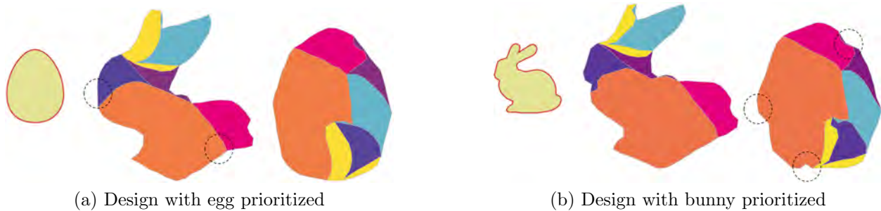
Figure 7.4: A failure. The input shapes are shown in gold. Even with user interaction, problematic regions (circled) in both shapes cannot be eliminated in a single design.
