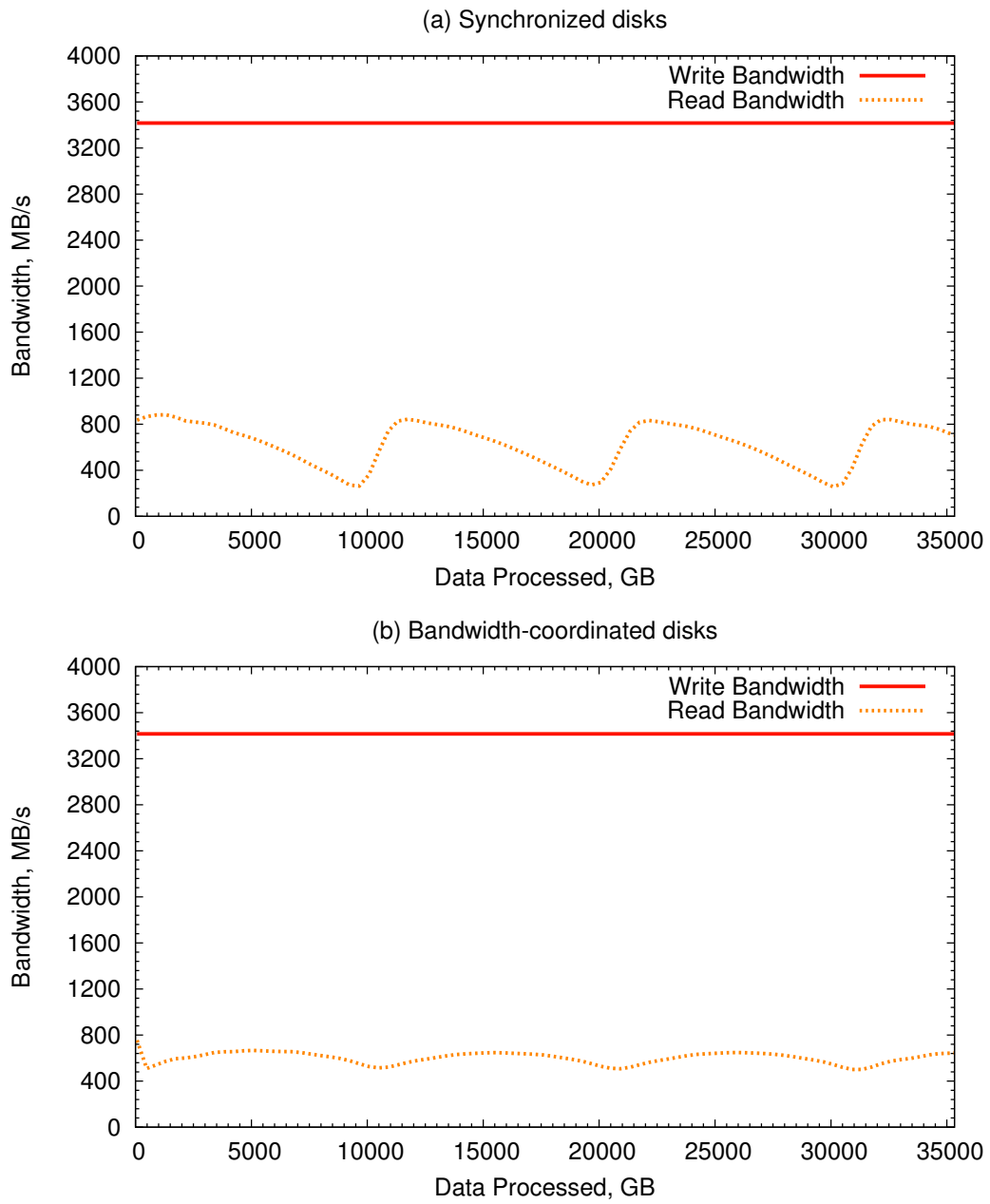
Figure 6.7: Valmar large-scale operation. This graph shows the results of coordinated Valmar processes running on 69 disks over 24 storage nodes with two different methods of disk coordination.
