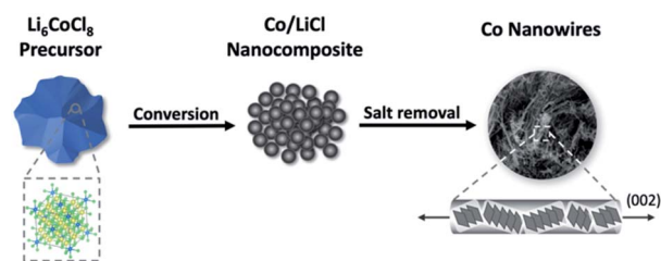
Fig. 1 Schematic of synthesis procedure for producing Co NWs. \text{Li}_6\text{CoCl}_8 first undergoes a conversion reaction with n -BuLi to form a nanocomposite, from which the salt is removed to leave Co NWs.
