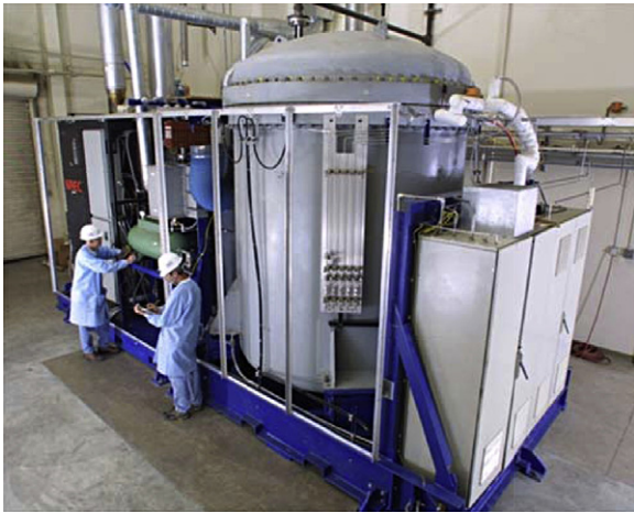
Fig. 1. Pressurized 220 kW SOFC/GT hybrid system.
