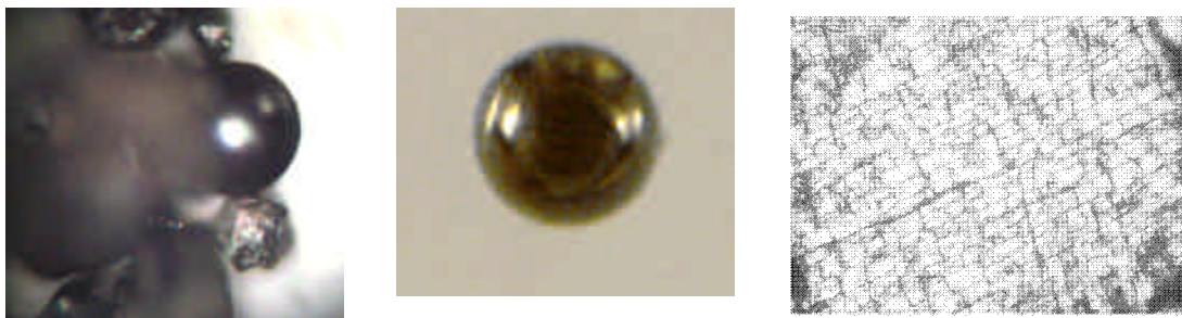
FIGURE 1. Magnetic particles from the Gainey MI site. Shown are a black, highly magnetic particle, a translucent perfectly spherical particle, and a thin slice with a rhombohedral cleavage pattern that is consistent with an explosive shock.
