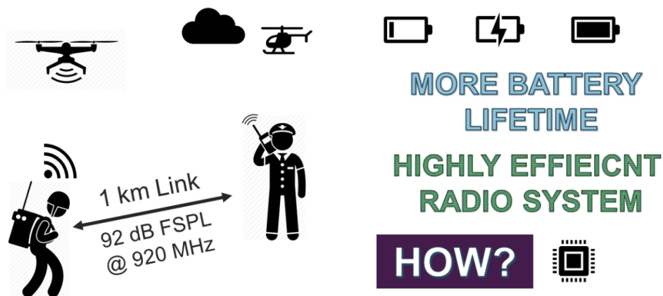
Figure 2. Existing problem for long range low power radio communication.
