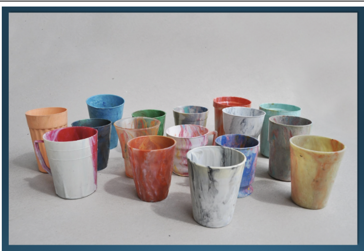
Recycled Cups in Cuba, made by mixing plastic from various sources. Resolviendo Archival photo. Photo by Ernesto Oroza
