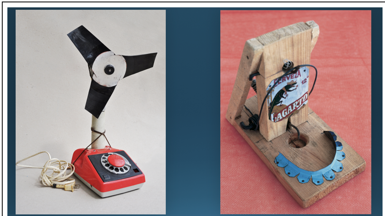
Soviet “Orbit” fan repaired with telephone components and a vinyl disc as blades, next to a Guillotine mousetrap made from wooden base, metal spring, and pieces of a beer can. Both cataloged in Cuba by Ernesto Oroza, left 2007, right 1999 (with Penelope de Bozzi)
