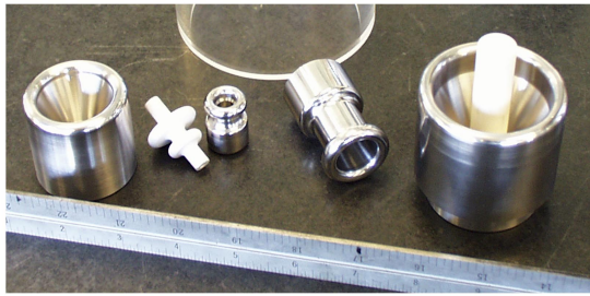
Figure 5. Insulator standoffs prior to testing. Shown are (left) the chopper to ground (G5-G4) insulators, and (right) the main insulator (main support to -65 kV source potential)
