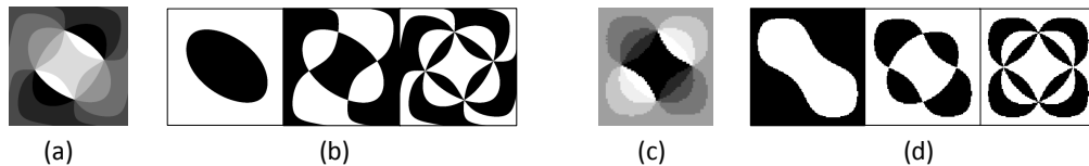
Fig. 5. Compressed ( 2^N ) lithography masks for fabricating multi-phase MFGs from fused silica (glass) wafers. Multiple etch rounds use the different masks to successively shape the MFG patterns. (a) Multi-phase grating function for nine-plane MFG calculated using the pixelflipper algorithm [2]. (b) Lithography masks for manufacturing the eight-layer pattern in a , compressed into N = 3 masks ( 2^3 = 8 ) with active areas that partially overlap during the three successive etch rounds. (c) Multiple solutions to a desired energy distribution are sometimes found during grating function design. For example, this pattern provides an intensity distribution that is effectively identical to that of the pattern in a . By exploring different shapes and different layer orders one can find patterns suited for the manufacturing process. (d) Lithography masks for the pattern in c .
