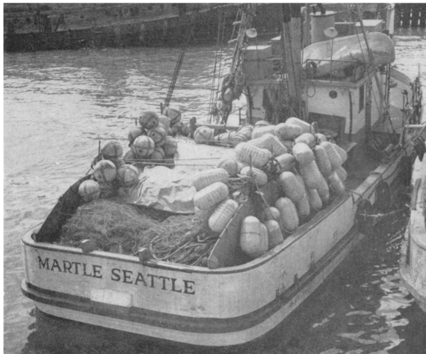
FIGURE 2. A shark vessel with a drift gill net stacked in the net bin
