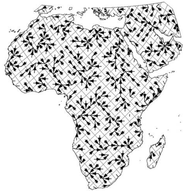
Figure 9. Upscaled African river network developed with the DMM, with coarse-resolution grid rotated 45°.
