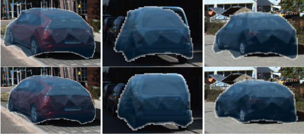
Figure 4.11. Top: category-level model before shape optimization. Bottom: instance-level model after shape optimization.
