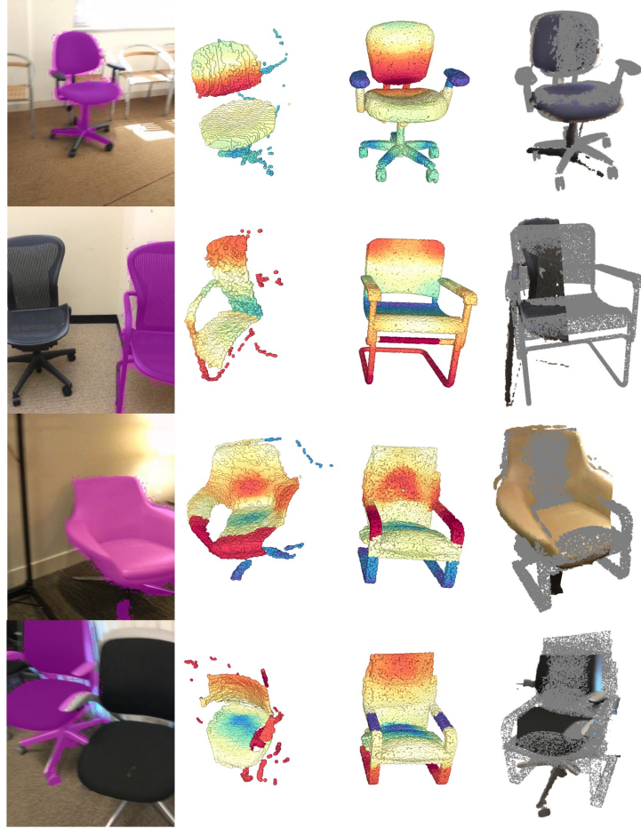
Figure 3.13. Examples on matching the point cloud segmented from a single RGB-D image from ScanNet dataset [34]. Column 1: RGB images and object segmentation masks in purple. Column 2 & 3: color-coded point cloud features of the observed objects and the CAD models. Column 4: Alignment results with the CAD models painted in grey.
