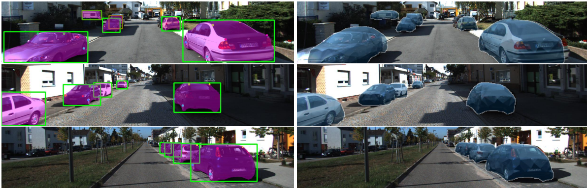
Figure 4.10. Left: the semantic observations. Right: the projection of reconstructed mesh models.
