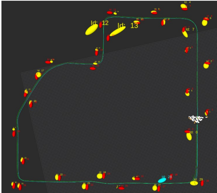
Figure 4.13. OrcVIO on simulation dataset. The red ellipsoids are the groundtruth objects. The yellow ellipsoids are the estimated objects. The cyan ellipsoids are the estimated outlier objects. The cyan line is the groundtruth trajectory. The green line is the estimated trajectory.
