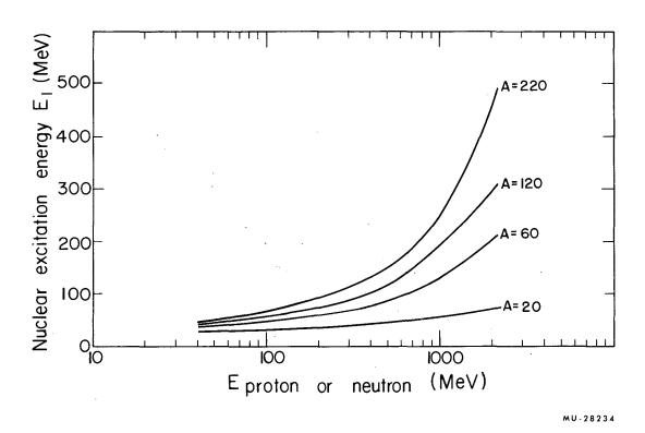
Fig. 11. Average nuclear excitation energy E<sub>1</sub> deposited in nucleus A by an incident neutron or proton of energy E in one inelastic collision.
