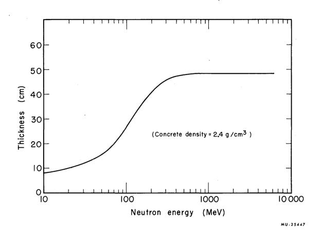
Fig. 3. Half-value thickness for high-energy neutrons in ordinary concrete.
