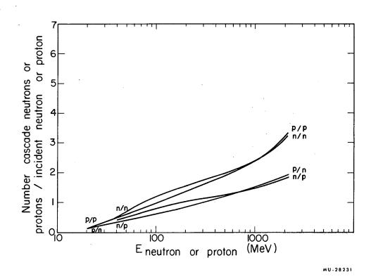
Fig. 2. Estimated <u>cascade neutrons</u> and <u>protons</u> produced by incident neutrons or protons of energy E<sub>n</sub> on nuclei near A = 20 per incident particle per inelastic collision. From Metropolis et al. (reference 4).
