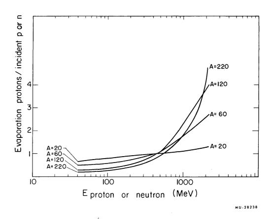
Fig. 17. Average number of evaporation protons per incident proton or neutron on various A's per inelastic collision vs energy of the incident particle, from Metropolis et al. (reference 4).
