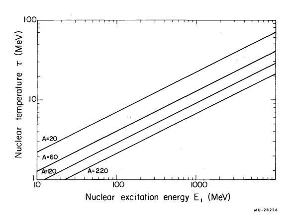
Fig. 13. Nuclear temperature  $\tau$  vs nuclear excitation energy  $E_1$  for various A's.
