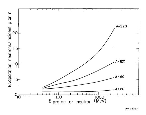
Fig. 14. Estimated number of evaporation neutrons produced per incident neutron or proton of energy E per inelastic collision, from Metropolis et al. (reference 4).
