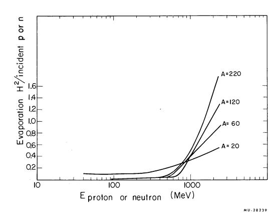
Fig. 18. Average number of evaporation H<sup>2</sup> per incident proton or neutron on various A's per inelastic collision vs energy of the incident particle, from Metropolis et al. (reference 4).
