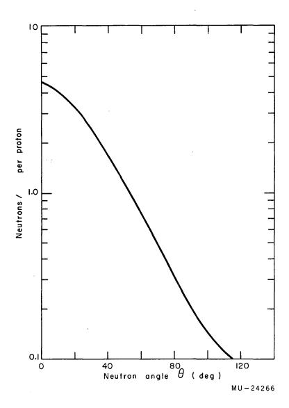
Fig. 8. Angular distribution of neutrons, over 150 MeV in energy, from a single collision in Cu by 6.3-GeV protons (normalized to 8 neutrons/proton), from Metropolis et al. (reference 4).
