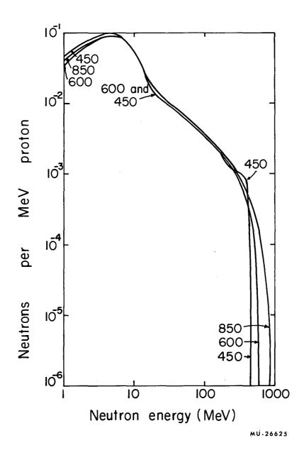
Fig. 7. Cascade and evaporation-neutron emission spectra from 450-, 600-, and 850-MeV protons on aluminum, per incident proton.
