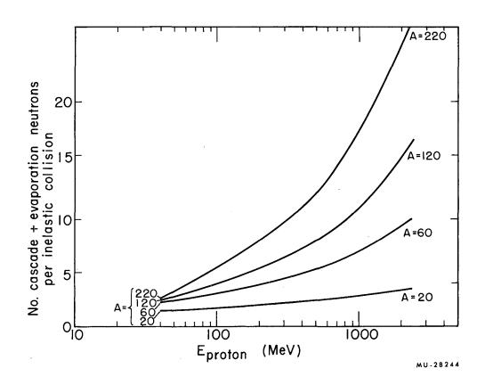
Fig. 15. Total neutron production per inelastic collision = cascade + evaporation as a function of the incident proton energy.
