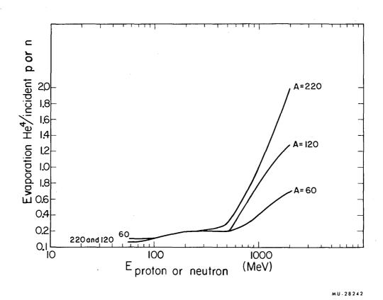
Fig. 21. Average number of evaporation He<sup>4</sup> per incident proton or neutron on various A's per inelastic collision vs energy of the incident particle, from Metropolis et al. (reference 4).
