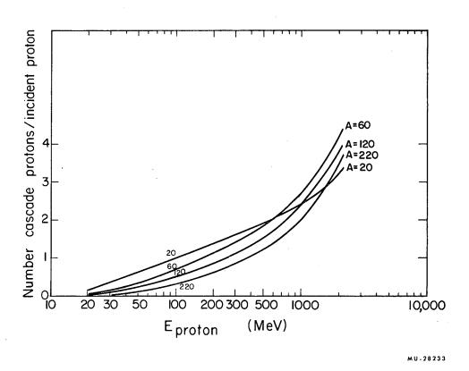
Fig. 10. Number of <u>cascade protons</u> per incident proton per inelastic collision as a function of proton energy and target A, from Metropolis et al. (reference 4).
