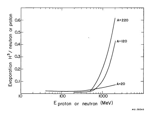
Fig. 19. Average number of evaporation H<sup>3</sup> per incident proton or neutron on various A's per inelastic collision vs energy of the incident particle, from Metropolis et al. (reference 4).
