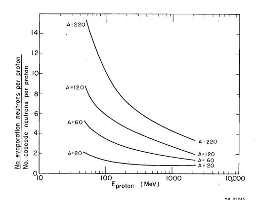
Fig. 16. Ratio of evaporation neutrons to cascade neutrons per inelastic collision as a function of the incident proton energy.
