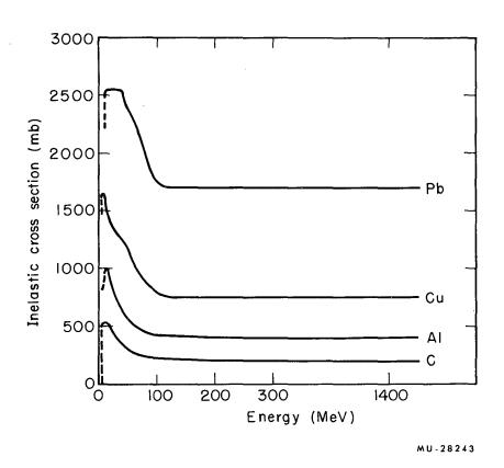
Fig. 9. Neutron or proton inelastic cross sections for C, Al, Cu, and Pb vs incident neutron or proton energy, from Lindenbaum (reference 5).
