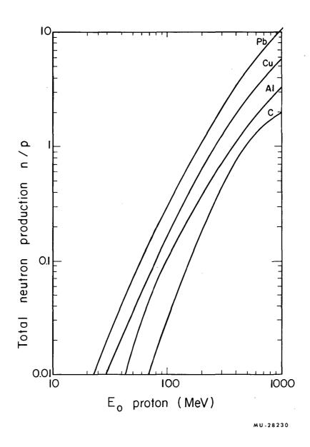
Fig. 1. Measured total neutron yields per proton stopping in a thick target for C, Al, Cu, and Pb. From Moyer (reference 2).
