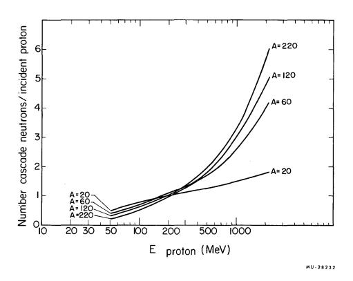
Fig. 6. Number of <u>cascade neutrons</u> per incident proton per inelastic collision as a function of proton energy and target A, from Metropolis et al. (reference 4).
