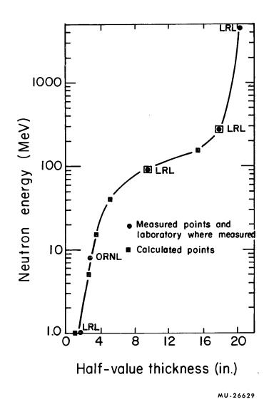
Fig. 4. Attenuation of neutrons in ordinary concrete. At 90 and 270 MeV, measurements were made at the 184-inch 340-MeV cyclotron. At 4.5 GeV the measurement was made at the Bevatron.
