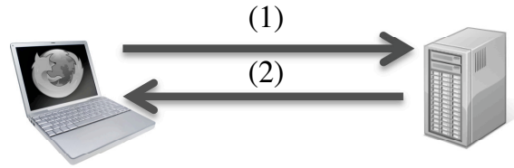
Figure 1.1: Example interaction between a web browser and a web server. In (1), the web browser makes an HTTP request to the webservice, and in (2) the web server sends the web browser an HTTP response containing the HTML of the web page.
