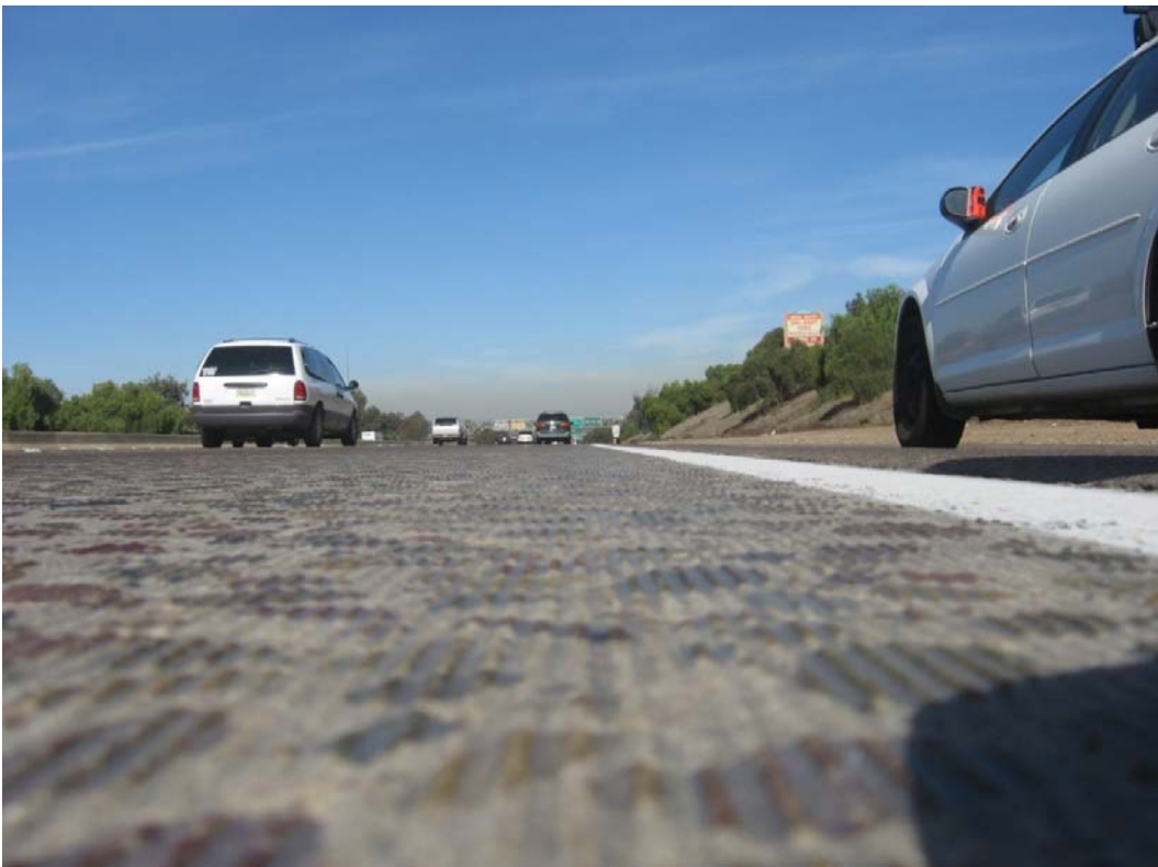
Figure A.4: Diamond ground, OBSI=107.2 dB(A) (Section QP-132.2).
