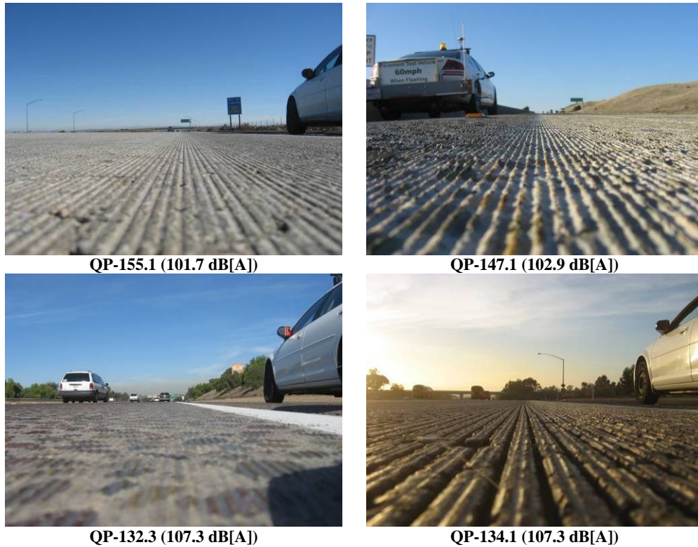
Figure 4.2: Example photographs of diamond ground surfaces and their OBSI levels.
