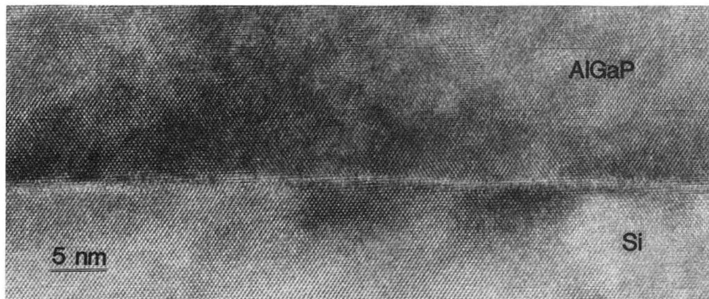
Figure 11 For growth of GaP on Si it has been shown that addition of small amounts of Al promotes perfect layer by layer growth resulting in very few defects compared to the more typical island growth mode. (XBB 894-3163)
