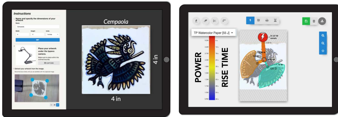
Figure 7.8: Capturing a Thermoreactive Composition. An image is transferred through a network connected camera, processed through the web app, and transferred to form the backdrop of the design canvas.
