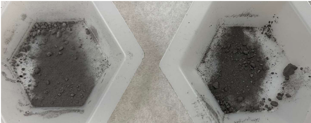
Figure 6.2. Stored vs non-stored amalgam. Image width: ~3in or ~7.6cm. Left: 10wt%eGIS-90wt%Al amalgam at 6 months of storage. Right: a different amalgam of same composition at less than one day of storage.
