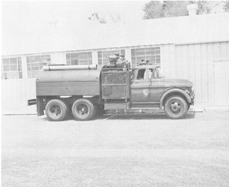
FIGURE 47. 1,500-gallon fish transport truck. Electric aeration and refrigeration equipment is driven by generators mounted at top of mechanical compartment. Photograph by Harold Wolf, July, 1958.
