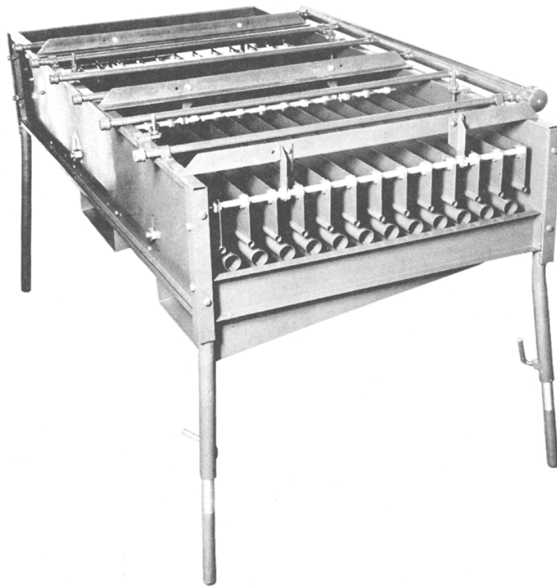
FIGURE 43. Morton adjustable fish grader. Photograph by Sartorius Company, Inc., San Francisco, California.
