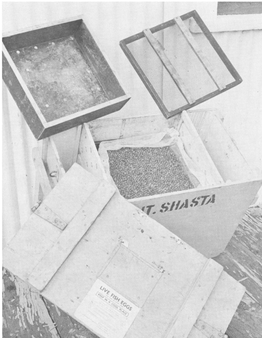
FIGURE 25. Lightweight egg shipping case made of marine plywood. Egg trays are made of 1 in. x \frac{1}{2} in. wood molding, covered with common window screen and painted with asphaltum varnish. Bottom tray shown in upper right of picture is turned bottom side up to show the two wood cleats which hold the tray up from the bottom of the case. Egg trays are 14 in. x 14 in. x 1 in. and will hold 70 ounces of eggs regardless of the number per ounce. The case holds 20 egg trays. Both ends of the egg case and the top ice tray are filled with cracked ice before shipping. Melting ice in the ice tray drips down through the eggs, keeping them moist. Photograph by George Farnham, February, 1958.
