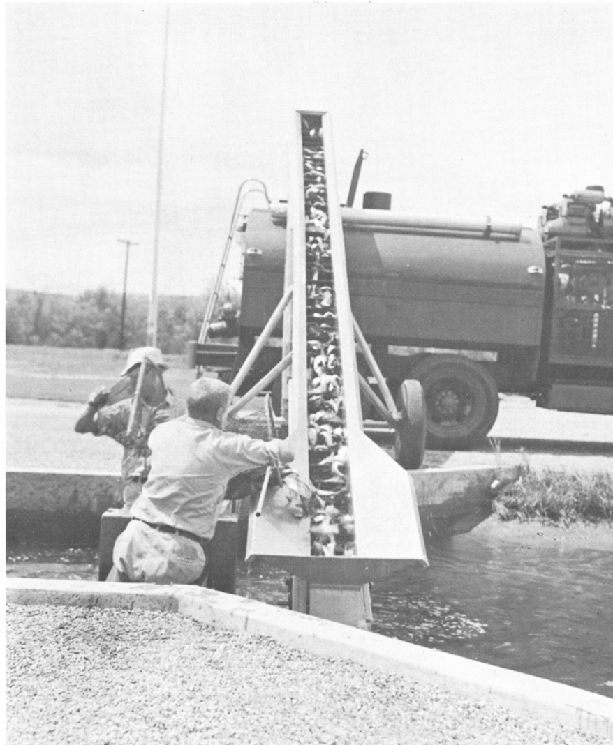
FIGURE 45. Fish loader for loading catchable-size fish into planting trucks. Displacement method of weighing fish is used. Sight gauge on back of truck is calibrated in increments of 50 pounds for accurate reading. Photograph by William M. Carah, May, 1956.
