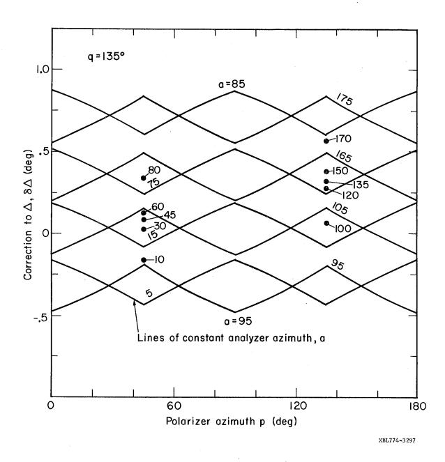
Fig. B2. Correction to  $\Delta$  due to component imperfections. Quarter wave compensator at 135°, specimen mispositioning error  $\delta\beta=0$ .
