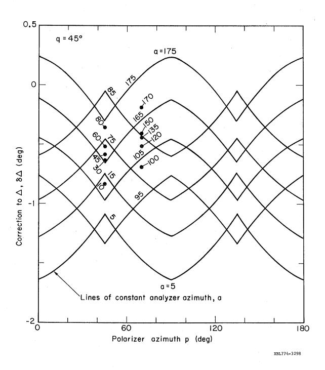
Fig. B1. Correction to  $\Delta$  due to component imperfections. Quarter wave compensator at 45°, specimen mispositioning error  $\delta\beta$  = 0.
