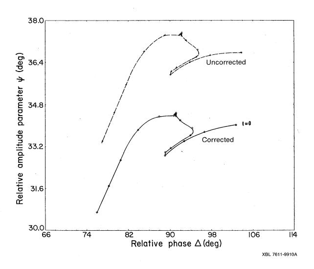
Fig. 4. Correction for ellipsometer imperfections Zn, 0.5M KOH, -1.0V vs. Hg/Hg0.
