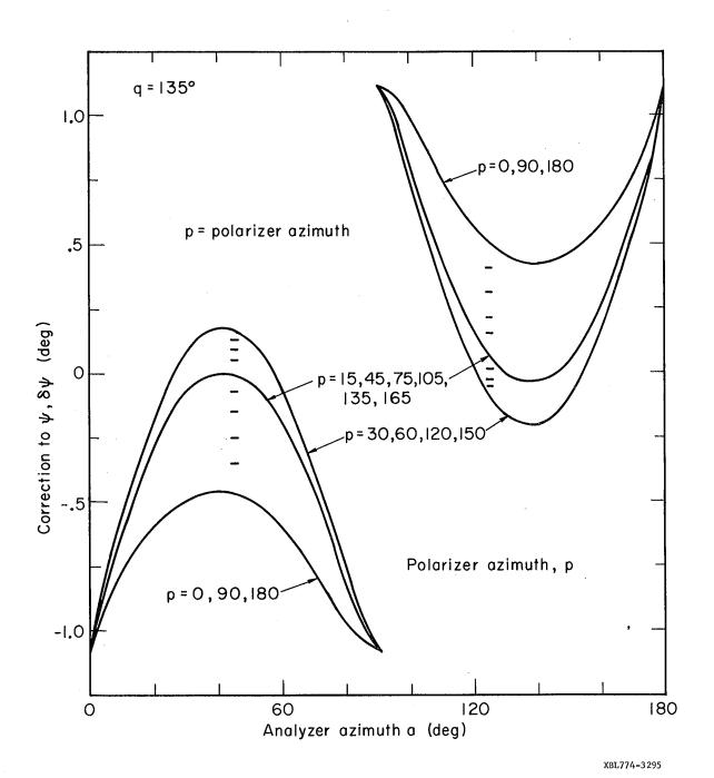
Fig. B4. Correction to  $\psi$  due to component imperfections. Quarter wave compensator at 135°, specimen mispositioning error  $\delta \beta = 0$  .
