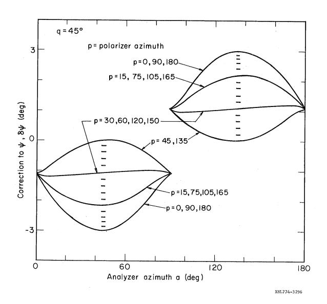
Fig. B3. Correction to  $\psi$  due to component imperfections. Quarter wave compensator at 45°, specimen mispositioning error  $\delta \beta$  = 0.
