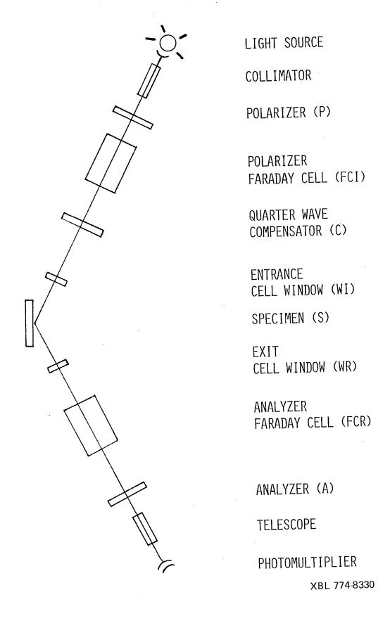
Fig. 1. Components of the automatic self-compensating ellipsometer.
