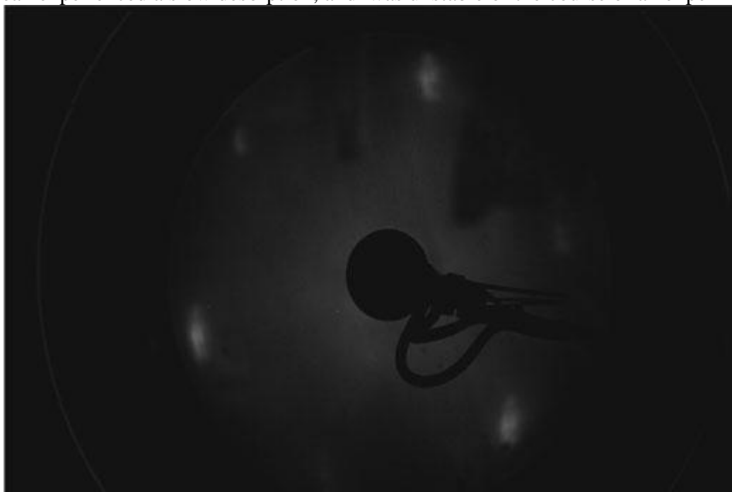
Figure 3.3 Low Energy Electron Diffraction of 1 monolayer toluene on Ag(111) taken at 71 eV. There are no spots visible for an ordered lattice of the toluene. The spots shown are diffraction from the underlying silver lattice. These spots are so large and misshapen because of the disordered nature of the toluene/silver interface.
