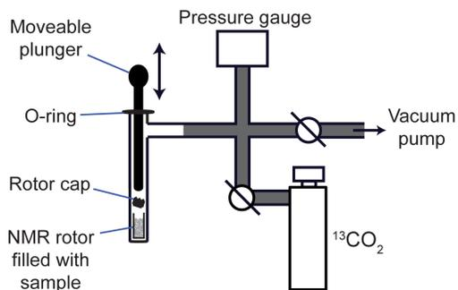
**Figure 2.** Schematic of home-built manifold for preparing gas-dosed NMR samples. The white section on the left is made from glass, and gray sections are made from stainless steel tubing. Swagelok® VCR metal gasket face seal fittings were used for steel-to-steel connections, and Swagelok® Ultra Torr fittings were used for glass-to-steel connections. Capacitance Manometers (MKS Instruments model 722B) were used for pressure measurements.
