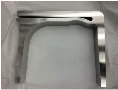
Figure 8: Tuner arm after UHV cleaning.
