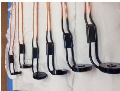
Figure 4: TiN coating of the coupling loop
