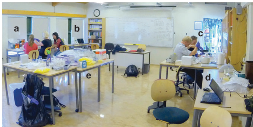
FIG. 3. The field lab during processing of Fimmvörðuháls samples: (a) DNA extraction, (b) qPCR, (c) nucleic acid staining, (d) ATP luminescence, (e) shared sterile consumables. Stations not shown: sample prep (grinding) room, dark room for microscopy. ATP, adenosine triphosphate; qPCR, quantitative polymerase chain reaction.
