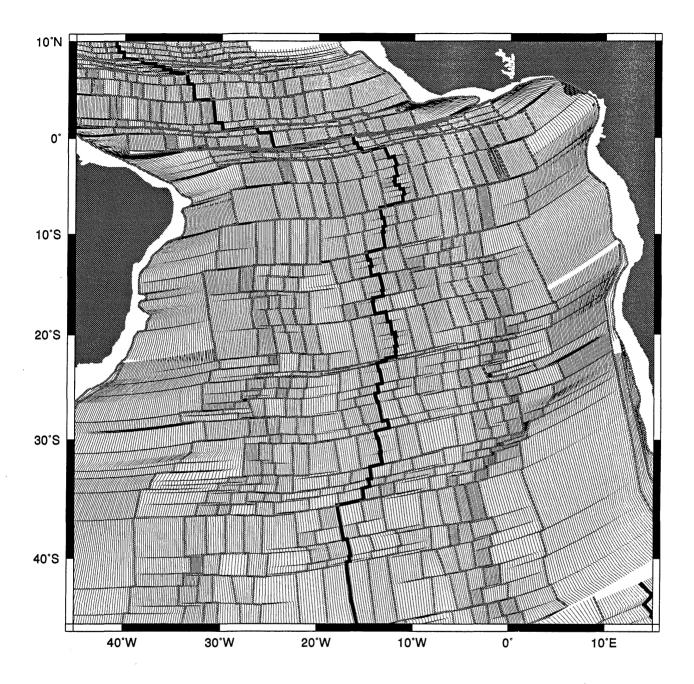
Fig. 1. Seafloor spreading isochrons in the South Atlantic, interpolated in 1 m.y. intervals. Broad grey lines delineate the isochrons bounding the individual interpolated stages. The isochrons correspond to magnetic anomalies 5, 6, 13, 18, 21, 25, 31, 34, M-0, M-4, M-10, M-16, M-21, M-25.
