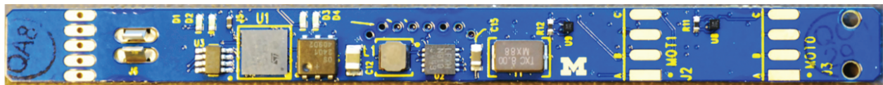
Figure 3.13: Electronics driver board for the fiber positioner, which was laid out at University of Michigan. On the left side is the spring clip which retains the fiber. On the right the two holes are where the board screws to the aft end of the positioner. The board is 8 mm wide and has been carefully designed so that all components, connectors, and fiber pass easily through the focal plate interface.
