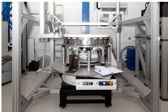
Figure 2.20: DECam C1 lens alignment setup.
