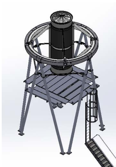
Figure 8.5: Extract from preliminary design for the lower of two Zenith work platforms, showing the stairs-plus-ladder access arrangement. Also shown, above the lower platform, are the braces for securing the upper Serrurier truss members when the top ring system is removed.
