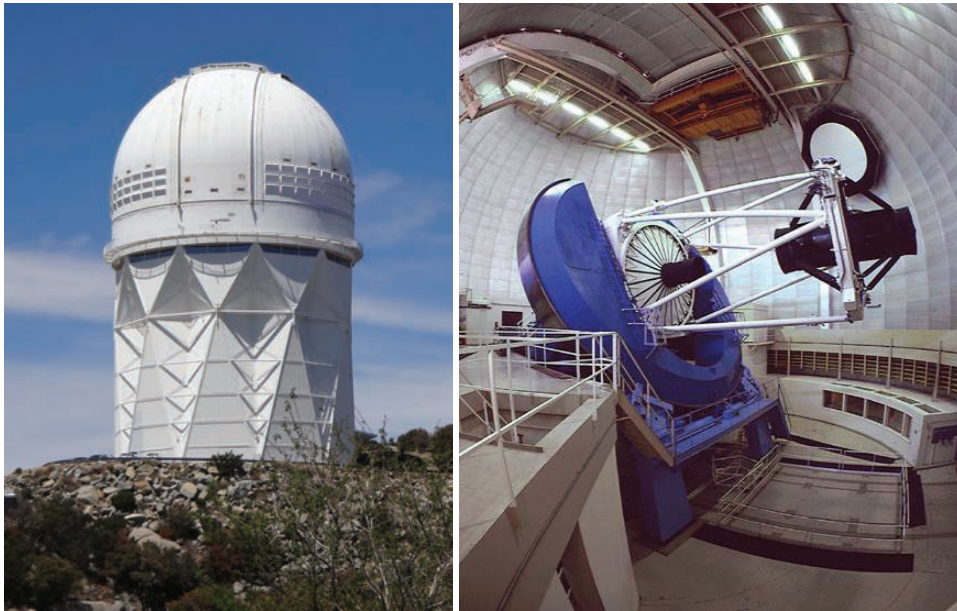
Figure 1.1: On the left is the Mayall 4m telescope dome structure. On the right is the telescope. The black cylinder is the MOSAIC corrector that will be replaced as part of the DESI project to instrument a 3 degree diameter field of view.
