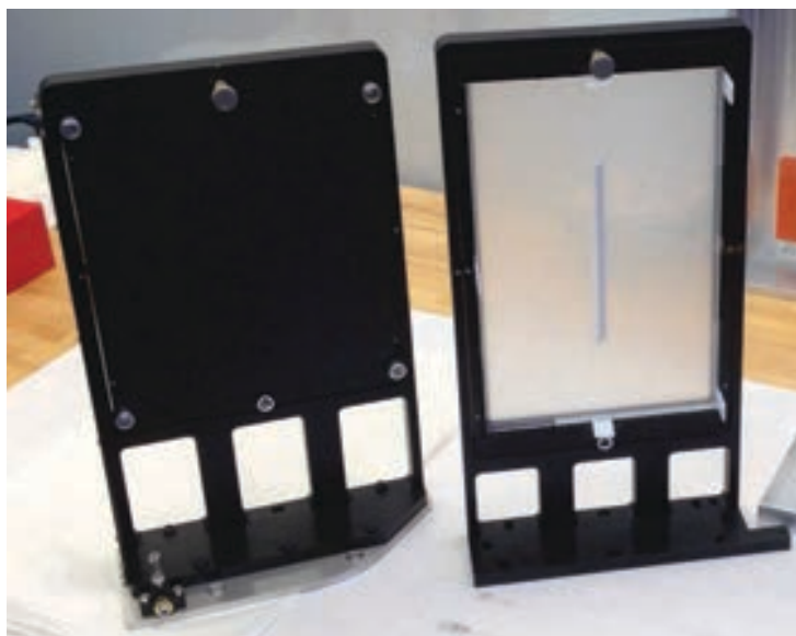
Figure 5.22: The mounts for the two dichroics. The one on the right has an uncoated substrate with a machined slot for fiber optic slit head to project light onto the collimator mirror.
