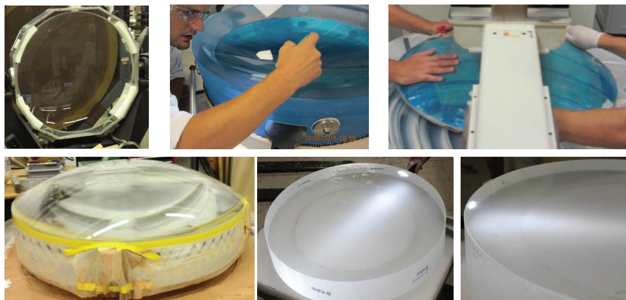
Figure 2.7: The six corrector lenses are shown in various phases of fabrication. From top left to bottom right: C1 C1 in transmission test, C2 concave (spherical) side being checked during final figuring, C3 convex surface being polished, C4 ready for final figuring, ADC1 blank, and ADC2 being machined.
