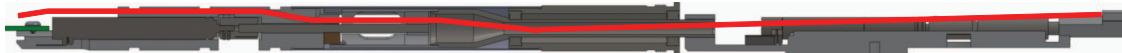
Figure 3.14: Fiber route through the fiber positioner is illustrated by a thick red line. Ferrule holder is at the right, exit at electronics board is on the left.
