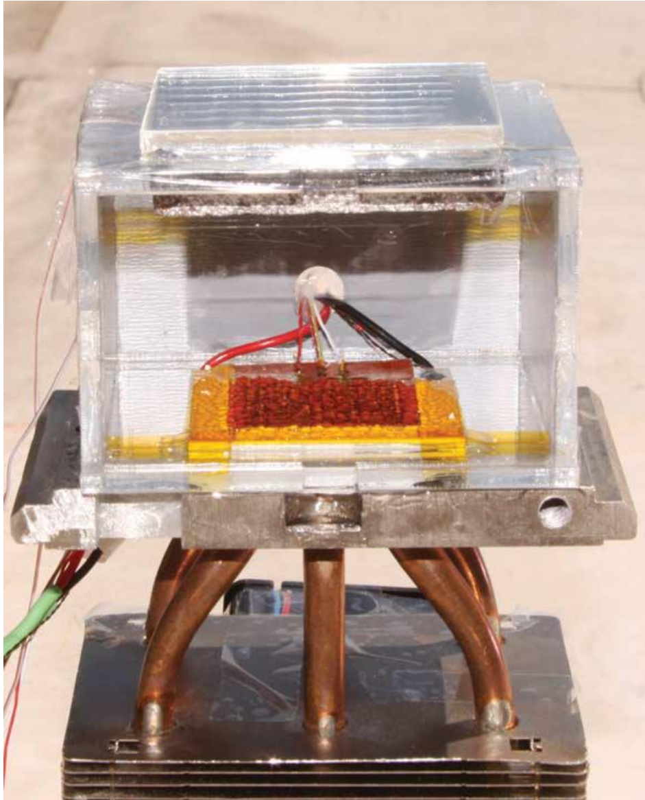
Figure 3. Image of a water-harvesting prototype with MOF-801[17]
