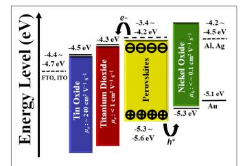
FIGURE 2 | Schematic illustrations of the energy bandgap of metal oxide charge transport materials and their carrier mobility (Jiang et al., 2018; Napari et al., 2020) in the bulk materials.
