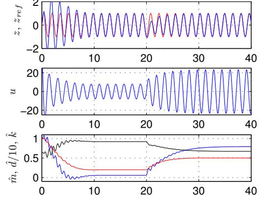
Fig. 6. Passivity based adaptive controller with single-DOF system. Top row:  $z$  (blue),  $z_{\text{ref}}$  (red). Bottom row:  $\hat{m}$  (blue),  $\hat{d}/10$  (red),  $\hat{k}$  (black).
