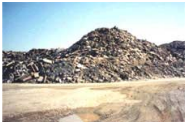
Figure 27. Stockpile of rubblized concrete.
