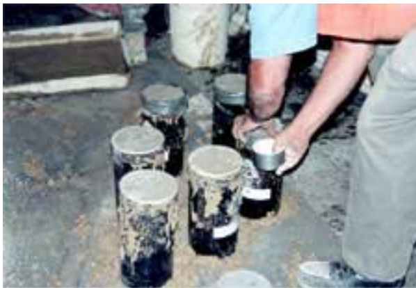
Figure 58. Six cylinder specimens were taken from every 15 mixer trucks for comprehensive testing.
