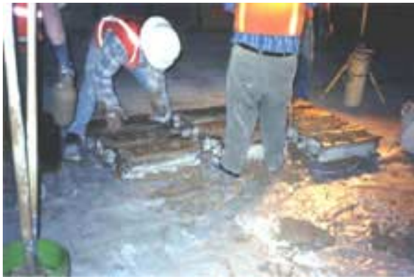
Figure 57. Ten beam specimens were taken from every 15 mixer trucks for flexural testing.
