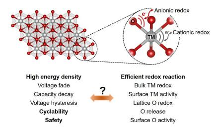
Figure 1. Schematic of the practical challenges and cationic-anionic redox reactions in
