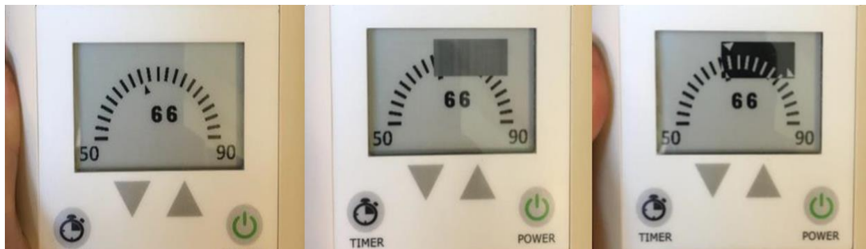
Figure 3. Setpoint change process on second hardware: setpoints disappear, then blinking box around new setpoint location, then reappearance of setpoints.
