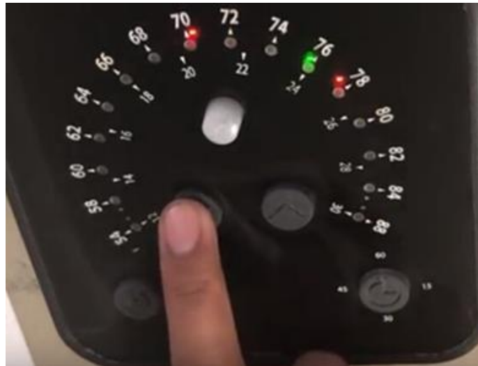
Figure 2. Labelled setpoints that change immediately upon user action on first hardware.
