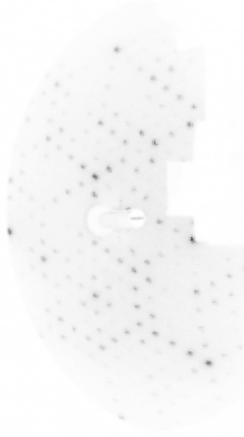
Figure 2.10: LEED image of clean, reconstructed Si(111)7 \times 7 surface.
