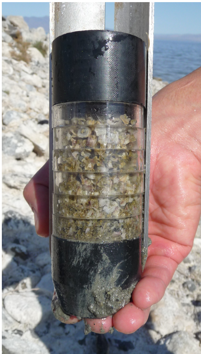
Figure 1. A core sample collected from Salton City shown to illustrate the abundance of barnacles in littoral sediment collected across a vertical depth gradient. Each ring has a depth equal to 2 cm (Photo: Juan Fernando Villa-Romero)
