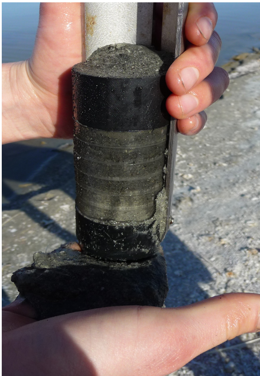
Figure 4. A view of the sediment core collected from site C. Each ring has a depth equal to 2 cm (Photo: Juan Fernando Villa-Romero)
