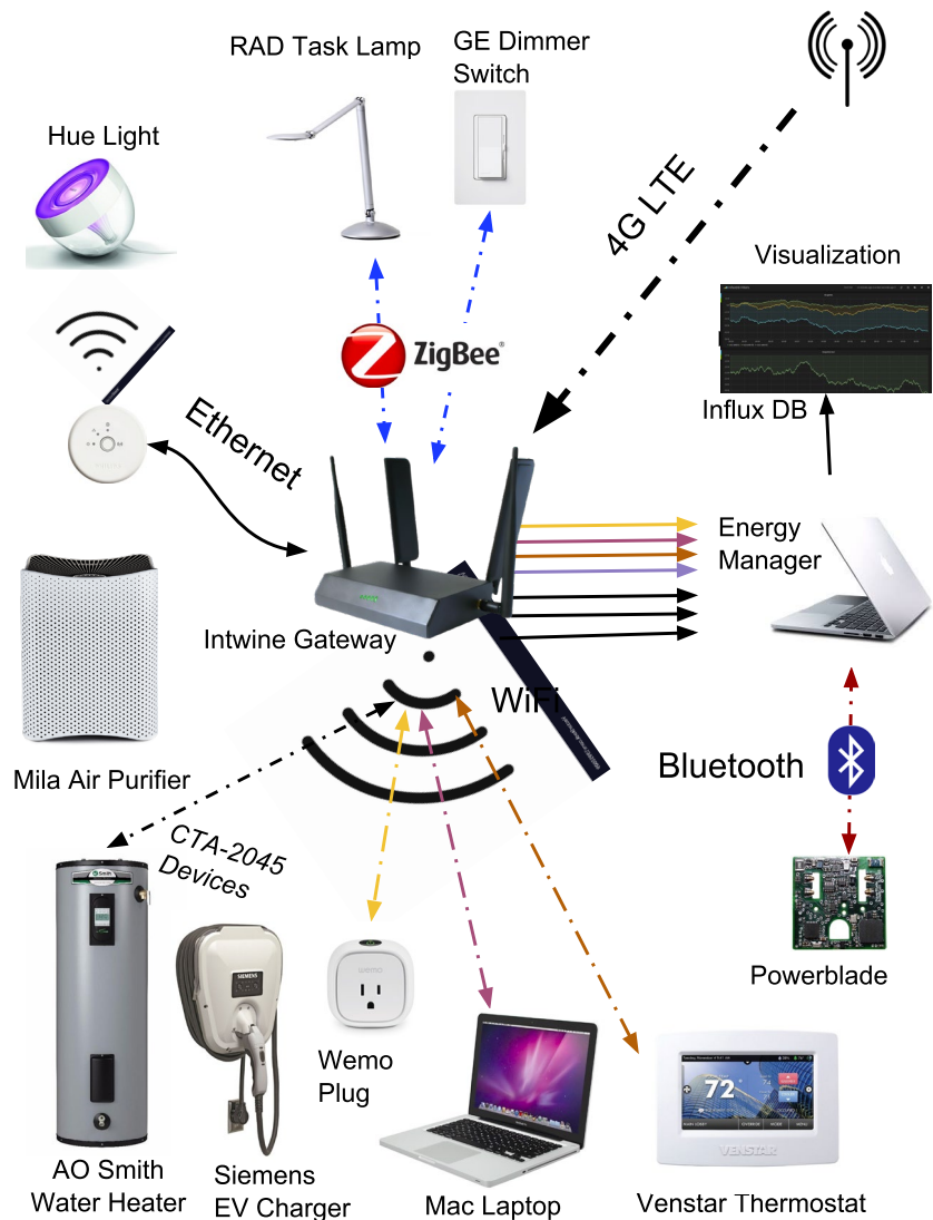
Figure 24: Demonstration Setup System Architecture
