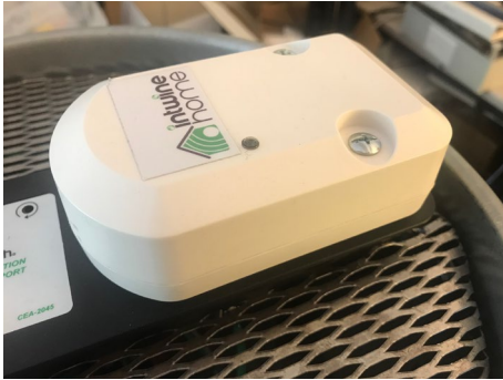
Figure 22: CTA-2045 Modules (AC and DC Form Factor)
