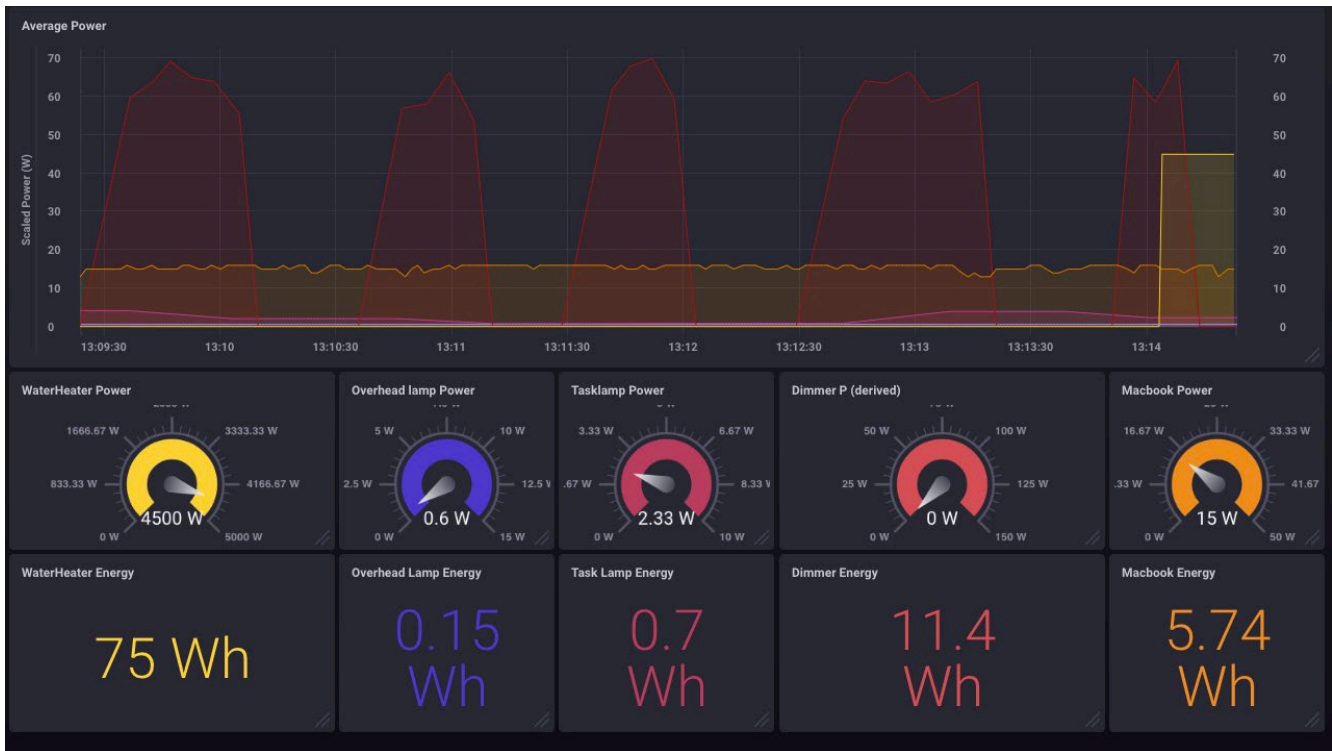
Figure 25: Snapshot of Energy Manager Dashboard Reporting Power and Cumulative Energy Consumption for Five Devices
