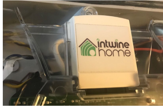
Figure 22: CTA-2045 Modules (AC and DC Form Factor)
