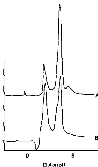
Figure 1. Chromatofocusing of 2 different samples of Fab17-IA. The line labeled A is the elution profile of Fab prepared from antibody purified with anion exchange chromatography, whereas line B represents Fab prepared from antibodies purified with protein G chromatography. The y-axis is absorbance in arbitrary units.
