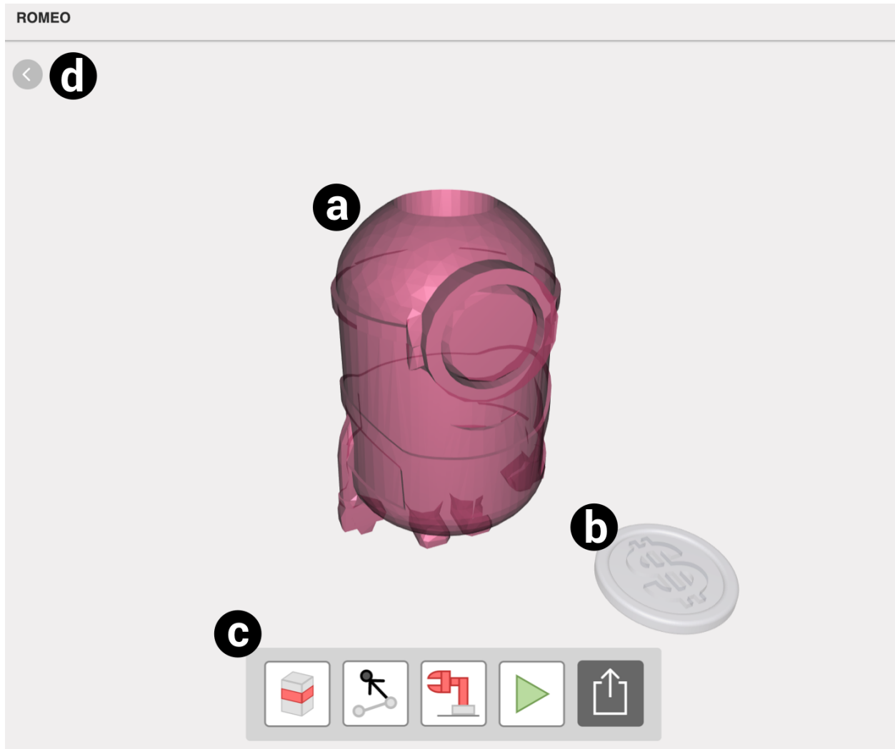
Figure 4.3: A screenshot of Romeo’s user interface: a) target object; b) reference object; c) functional buttons, from left to right: selecting transformable part, specifying motion points and action, generate embedded robotic arm, animation, export and d) button to restart the current step
