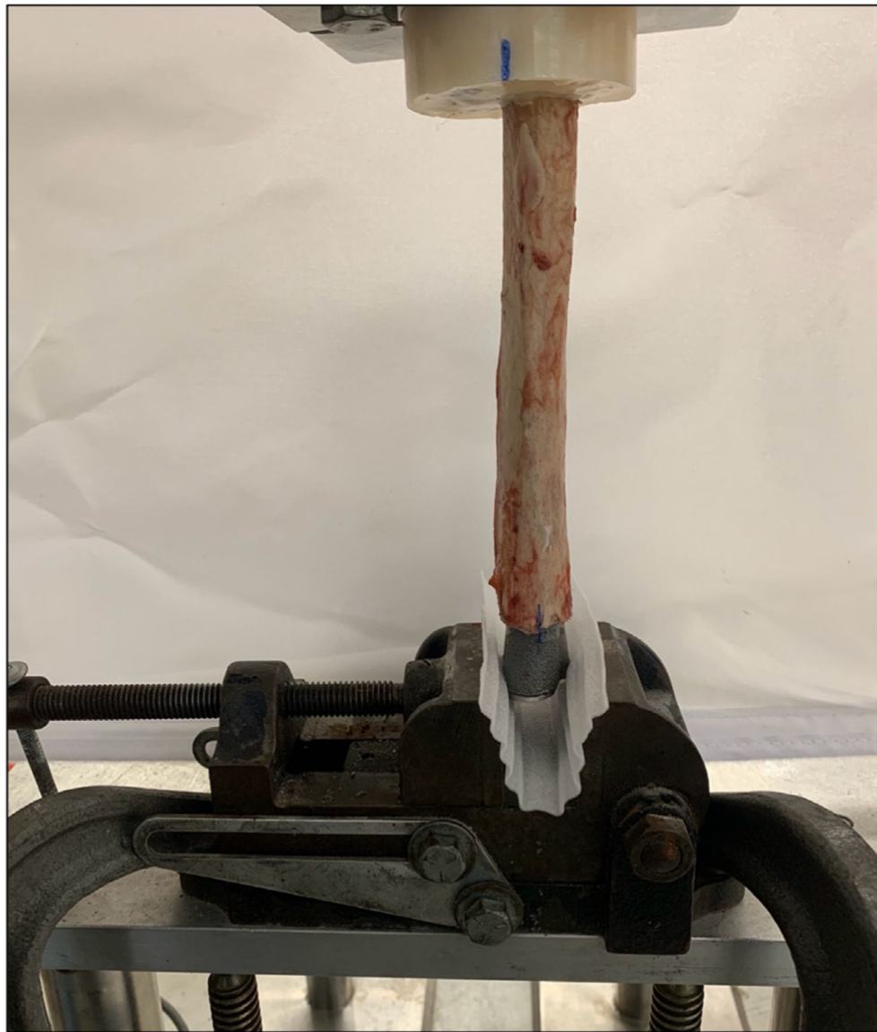
Figure 4. Torque tolerance testing setup with stationary vice capturing the humeral component. The humerus is potted in a PMMA cylinder, and the cylinder is attached to the KUKA robot, which applies progressive torque. PMMA , polymethyl methacrylate.
