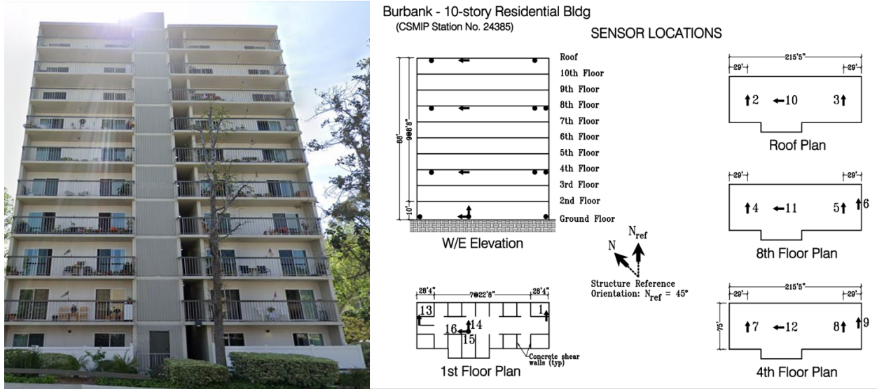
Figure 4.9. Side and plan view of CSMIP station.
