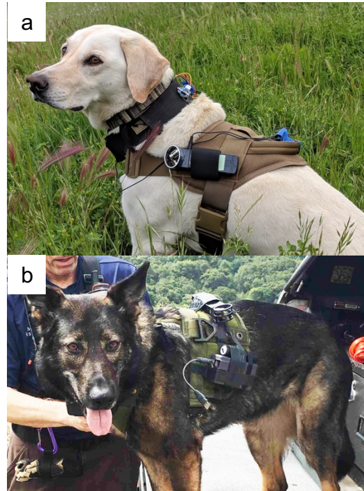
Figure 2.2. SAR dog wearing research harnesses. (a) Audio recorder, microphone collar, and tilt switch (blue chip attached to collar) are shown. (b) Data logger for GPS and tilt switch.
