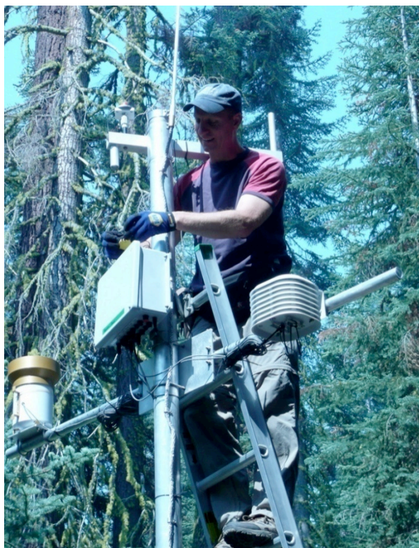
Figure 4: Hydro climate monitoring station
