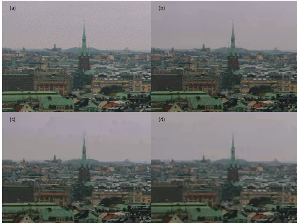
Figure 3.2: Examples of different encodings (1st frame from Old town sequence): (a) Original uncompressed frame, (b) Compressed at High rate, (c) Compressed at Low rate, (d) Filtered and Compressed at “On Stand” rate.
