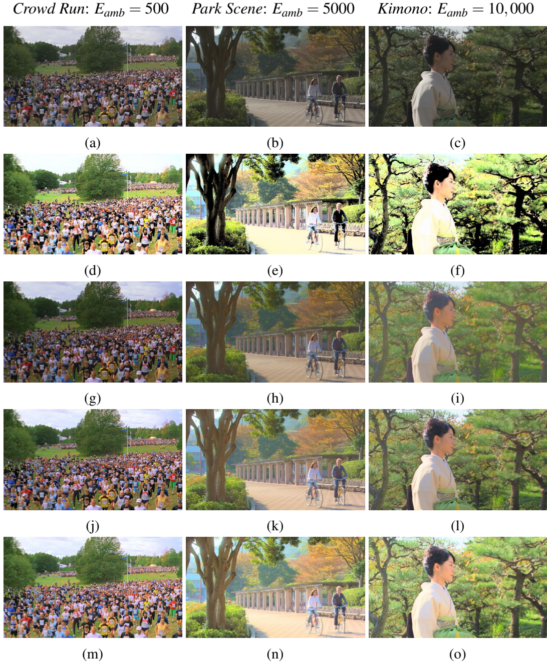
Figure 2.8: Images before and after tone mapping using different algorithms for L_W = 200 . (a) - (c): original; (d) - (f): Mantiuk et al. [15]; (g) - (i): Su et al. [20]; (j) - (l): proposed content independent enhancement; (m) - (o): proposed content dependent enhancement. Note that these are the inputs to the device, which do not show the look under the given ambient illumination.
