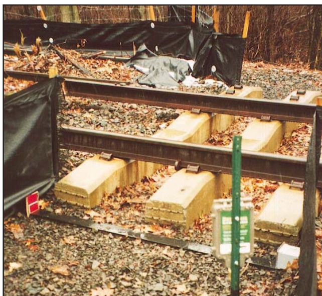
Photo 4. Infrared beam and reflector (flush with ground) triggers remote camera (foreground on post) when interrupted. Similar setups were positioned at each end of three crossing structures. Woodlot Alternatives, 2003.
