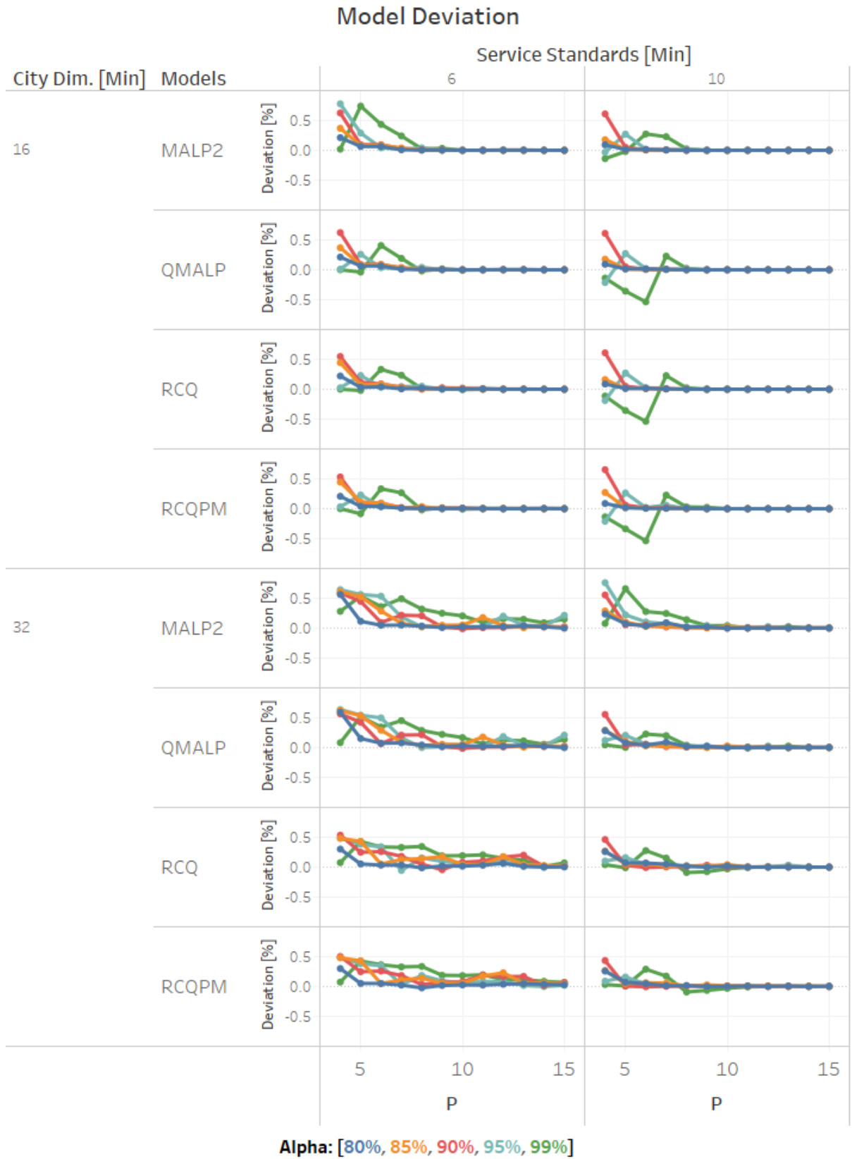
Figure 7 – Model deviation ( Predicted - Simulated reliability ) [%]: Low call intensity scenario (2 CPH)
